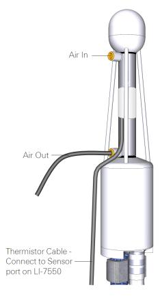
Figure 4-1. Flow calibration gas into the calibration fitting. Attach a 15 cm (6 in.) piece of tubing to the outlet to prevent diffusion of ambient air into the calibration fitting.
