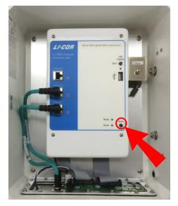
Figure 6-1. Reset button in the LI-7550.
