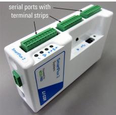
The SmartFlux 2 System comes standard with your analyzer and works with the LI-7550 Analyzer Interface Unit. It mounts inside a Biomet Enclosure, Systems Enclosure, or another suitable enclosure. This digital system includes a computer running EddyPro® software for on-site, real-time flux processing in an eddy covariance system.
